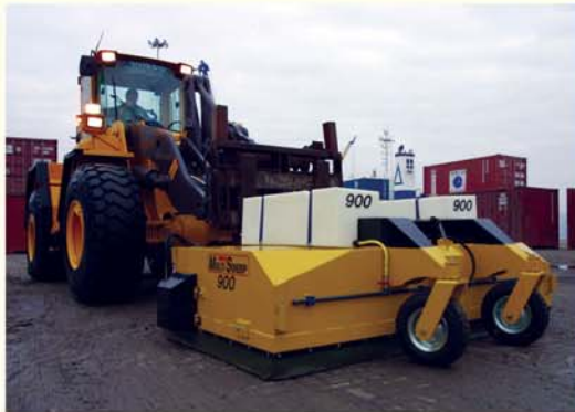
Model 900 complete with twin tank gravity water system.
