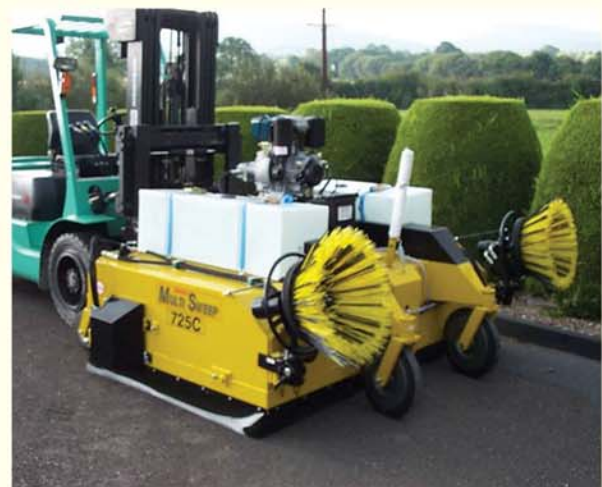
Model 725 complete with twin side brushes, gravity water system and powered by a diesel power pack.
